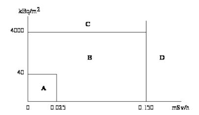
Figure 1. Zones determining equipment preparation for transport in the special vehicle
