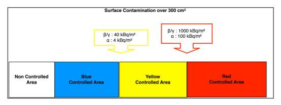
Figure 19. Criteria for the designation of controlled areas at the Ringhals nuclear power plant (surface contamination)
