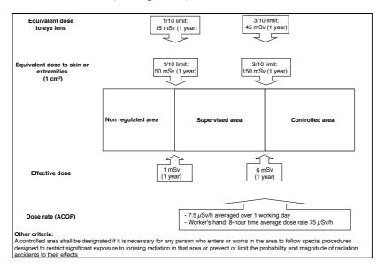
Figure 12. Criteria for the designation of supervised and controlled areas in the United Kingdom regulations
