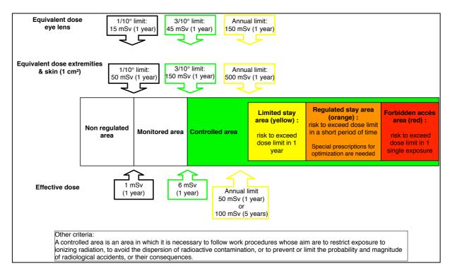
Figure 4. Criteria for the designation of monitored and controlled areas in the Spanish regulations
