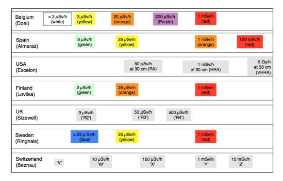
Figure 24. Dose rate criterion values for the designation of controlled areas the nuclear sector
