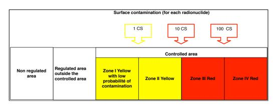
Figure 22. Criteria for the designation of regulated radiation areas in the Swiss regulations for nuclear facilities (surface contamination)
