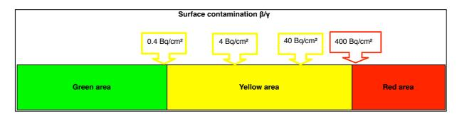
Figure 3. Criteria for the designation of controlled areas at the Doel nuclear power plant (surface contamination)
