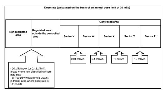
Figure 21. Criteria for the designation of controlled areas in the Swiss regulations for nuclear facilities (external exposure)
