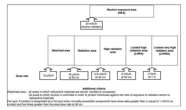
A location is designated as a hot spot when normally accessible components have dose rates greater than or equal to 1 mSv/h on contact and five times greater than the area dose rate at 30 cm.
