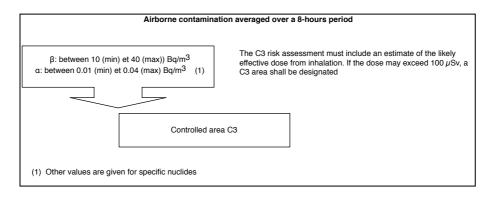
Figure 15. Criteria for the designation of controlled areas at the Sizewell nuclear power plant (airborne contamination)
