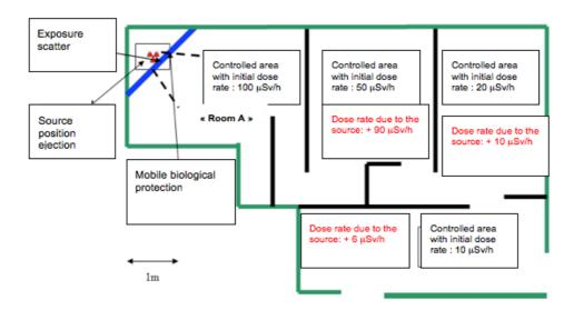
Comment: Below the rooms will be named room A (where the exposure takes place), west room (where the equivalent dose rate goes from 50 to 140 µSv/h during the exposure), east room (where the equivalent dose rate goes from 20 to 30 µSv/h during the exposure) and south room (where the equivalent dose rate goes from 10 to 16 µSv/h during the exposure).
