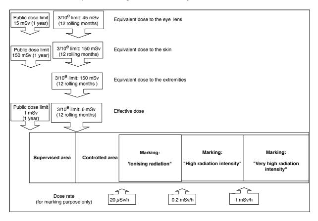
Figure 1. Criteria for the designation of supervised and controlled areas in Belgian regulations
