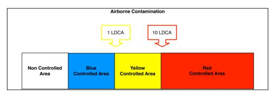
Figure 18. Criteria for the designation of controlled areas at the Ringhals nuclear power plant (airborne contamination)
