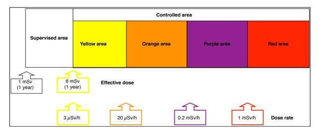
Figure 2. Criteria for the designation of supervised and controlled areas at the Doel nuclear power plant (external irradiation)
