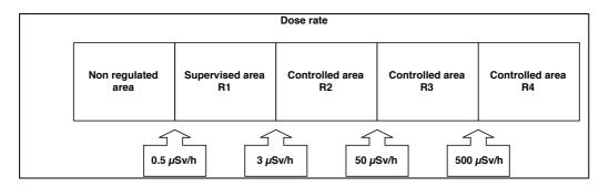
Figure 13. Criteria for the designation of supervised and controlled areas at the Sizewell nuclear power plant (external exposure)
